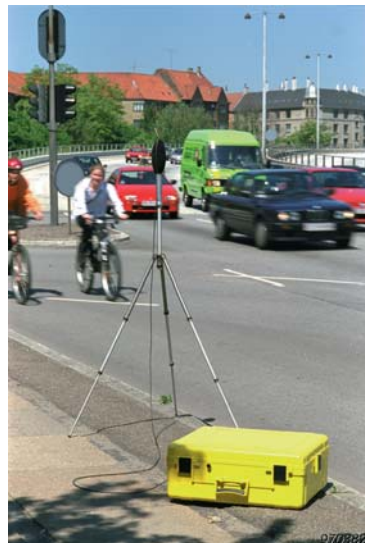
Fig. 9 Outdoor Gear Type 3592
