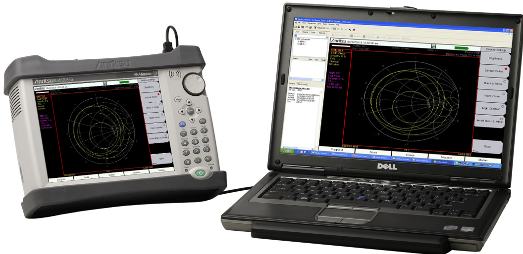
Figure 2-9. MS2035B Connected to PC via USB Mini-B
