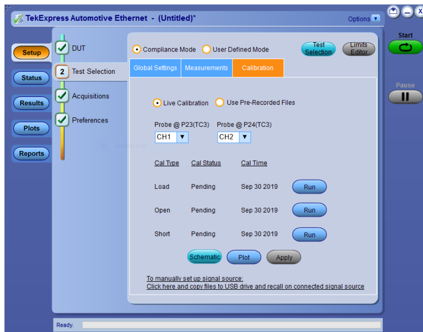
Figure 12: Calibration tab for return loss measurement
