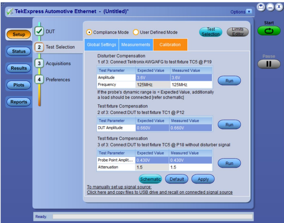
Figure 60: Calibration tab for 1000Base-T1 transmitter distortion measurement
