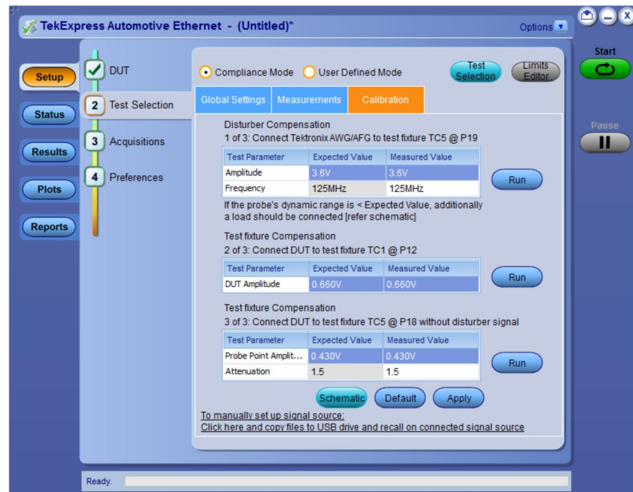
Figure 10: Calibration tab for 1000Base-T1 transmitter distortion measurement
