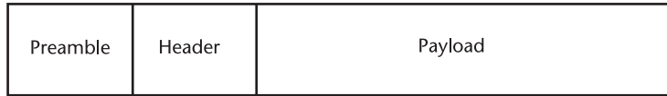
Figure 8.3 Common frame structure of wireless packet with preamble followed by header and payload data.
