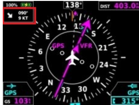
Figure 6-5 HSI Display of Crosswind (Typical Values Shown)
