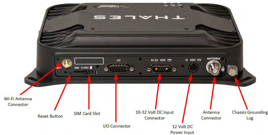
Figure 2-7 Terminal Unit (TU) Back Panel Detail
