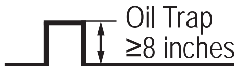
Figure 40: Close Up of An Inverted Oil Trap.
