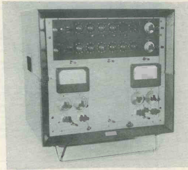
The Ekco automatic scaler type N610A for nucleonic work. The upper row of tubes performs the counting operation on the input pulses, whilst the lower row performs the automatic timing operations which enable the scaler to switch itself off after a pre-set time. The two tubes on the top right hand side of this scaler are not counting tubes; they are tubes for indicating the state of the count in two high speed valve counting circuits. (Ekco Electronics Ltd)
