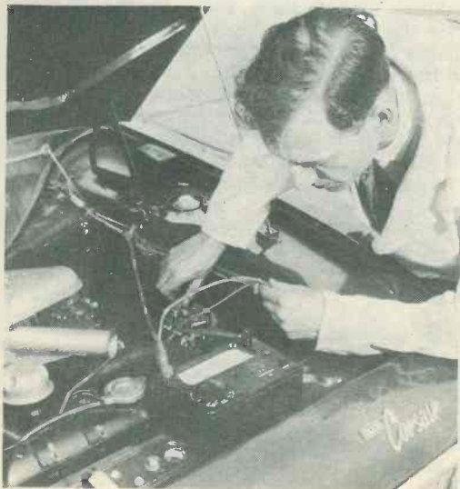
At the Dagenham factory of the Ford Motor Company, an engineer checks the open circuit voltage of a regulator on a Ford Consul Corsair using an AvoMeter Model 12. Avo is a member of the M.I. Group.
