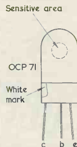
Fig. 5. Illustrating the lead-out connections and the sensitive area of the OCP71
