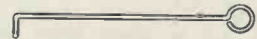
Fig. 4. A simple hook, fabricated from a cycle wheel spoke, which can be of considerable assistance when fitting tape recorder drive belts
