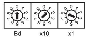
Internally, 1 is always added to the node number to avoid setting of the node number 0.
