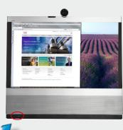
To start the system again, press the **Power** button until the LED illuminates (green light).
