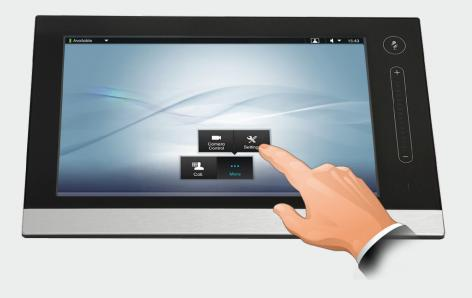
The EX90 can be configured via the touch screen controller or via its web interface. For full access to all configurable parameters the web interface must be used—the touch screen controller provides access to a limited set of parameters only.
