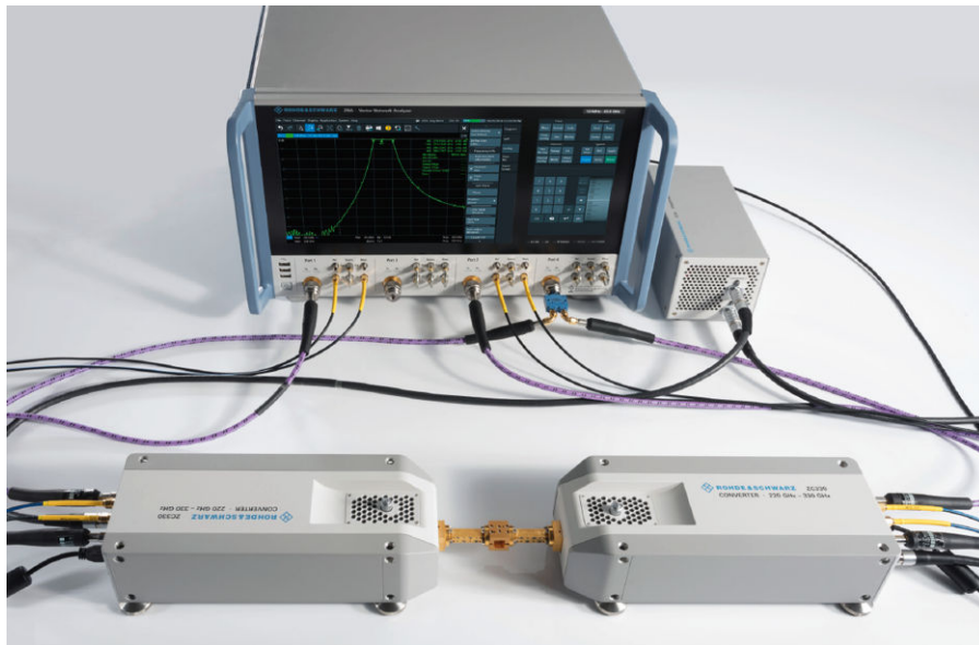
Figure 5-24: Frequency converter cabling: front connection
