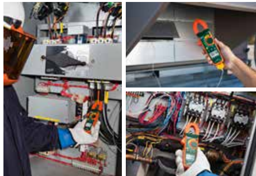
Troubleshoot current output on an electrical panel, verify Temperature output on HVAC units, and quickly detect live voltages with built-in Non-contact Voltage Detector.
