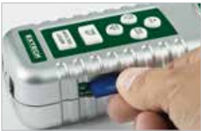
475040-SD & 475044-SD include SD memory card to conveniently datalog readings
