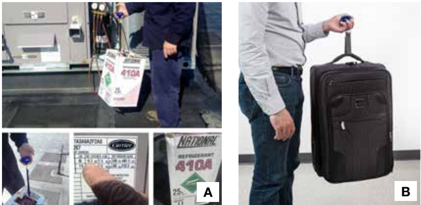
A. Verifying the level of refrigerant inside the tank as well as checking the remaining level when used before the next job. B. Conveniently weigh your luggage to ensure you meet the proper guidelines before checking your bag in at the airport.
