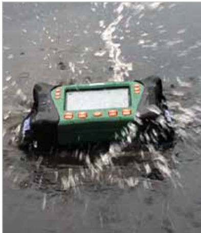
Drop-proof and Waterproof housing meets IP67 standards.
