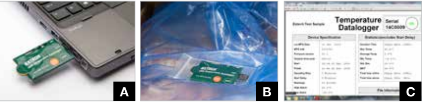
A. Plug into a PC to adjust the settings (requires Adobe® Reader® software) B. Put the Datalogger back inside plastic bag and seal the opening, then place in an area where temperature is to be monitored and press START for the unit to start recording C. When datalogging duration is completed, plug back into a PC where it will automatically generate a PDF report.
