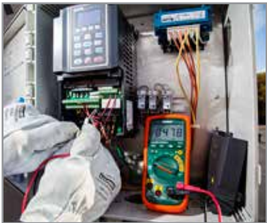
Low Past Filter (LPF) ensures accurate AC Voltage measurements on a variable frequency drive.
