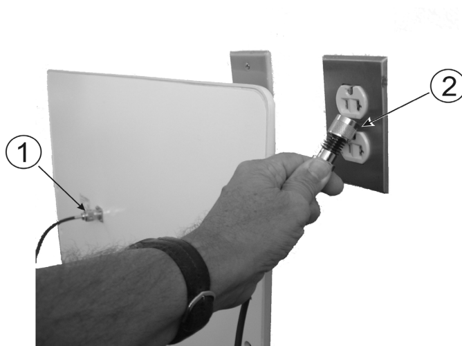
Figure 26 Short Load to Earth Ground
