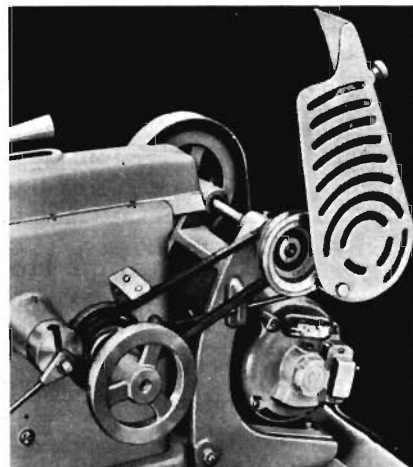
Guards on all belts and pulleys. Quick-acting belt tension release
