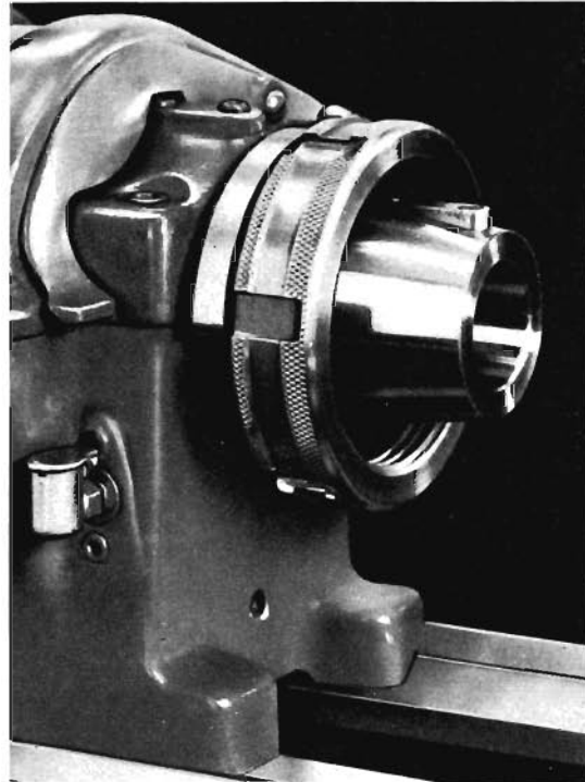
Size 00 Long Taper Key Drive Spindle
