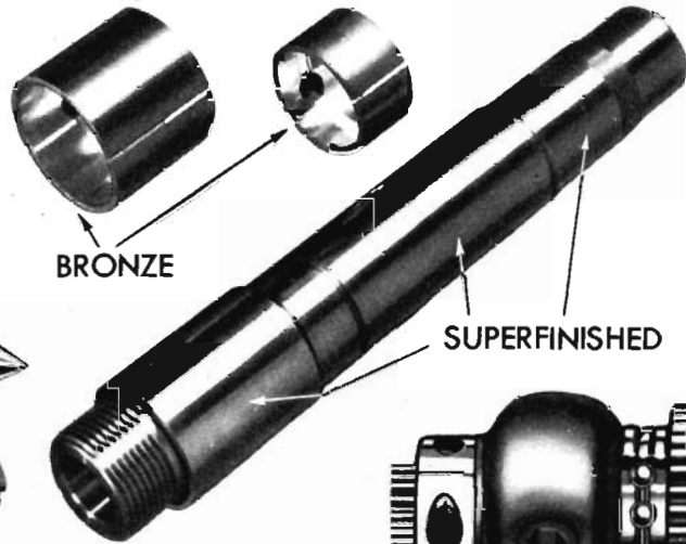
Fig. 17. Headstock Spindle and Bearings
