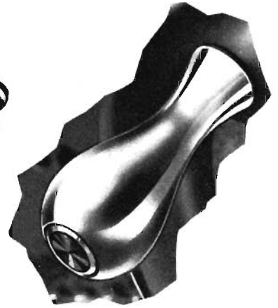
Fig. 23A. Close-up of Swivel Machine Handle on Apron Handwheel
