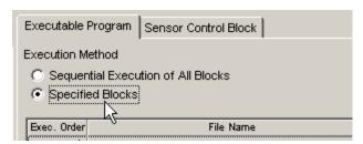
5. Program blocks are now added to the scan list. When "Specified Blocks" is selected, the first block (in this case, "MAIN") is always executed with other blocks executing only when activated.
