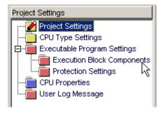
3. With the "Execution Block Components" dialog open, under the "Executable Program" tab, by default the "Execution Method is set to "Sequential Execution of All Blocks".
