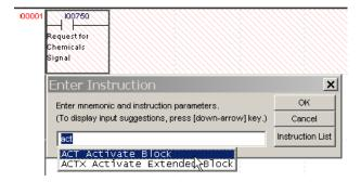
9. Enter "PUMPS" for the "Name of block to be activated" field. Then select "OK"
