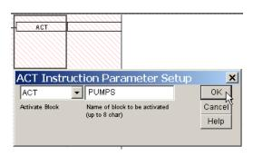
10. To allow for deactivation of the "Pumps" program block, another rung is added and the "NOT" condition of the "Request for Chemicals" signal is inserted at the beginning of the run and an "Inactive Block" application instruction is added to the rung...
