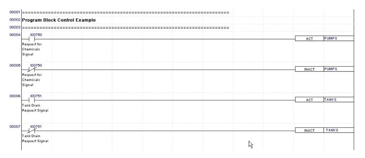
It is important to note that deactivating a block turns off all of the outputs in the block and for critical applications, due diligence should be exercised in the decision process concerning deactivating blocks.
