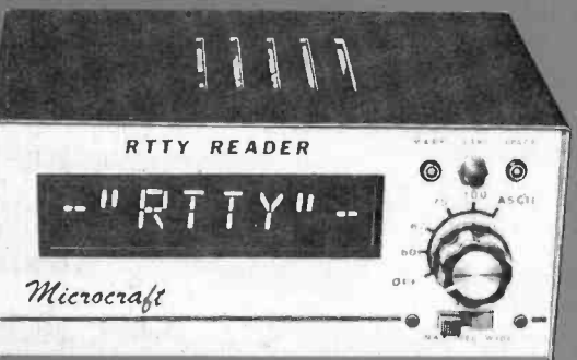
Microcraft's RTTY Reader uses a microprocessor to handle Baudot at four speeds or ASCII and display it on an eight-moving-character readout.
