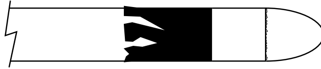
Figure 33. Torn catheter sleeve valve
