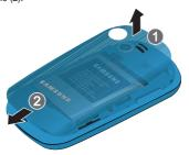
Lift the battery up (1) and away (2) from the phone, bottom end first
