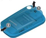
First, insert the top end of the battery (1), matching the gold contacts on the battery to those on the inside of the phone.
