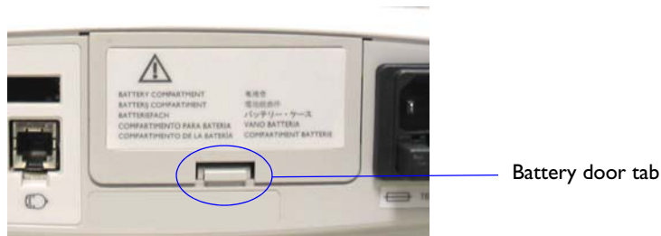
Figure 7-2 Removing the battery door
