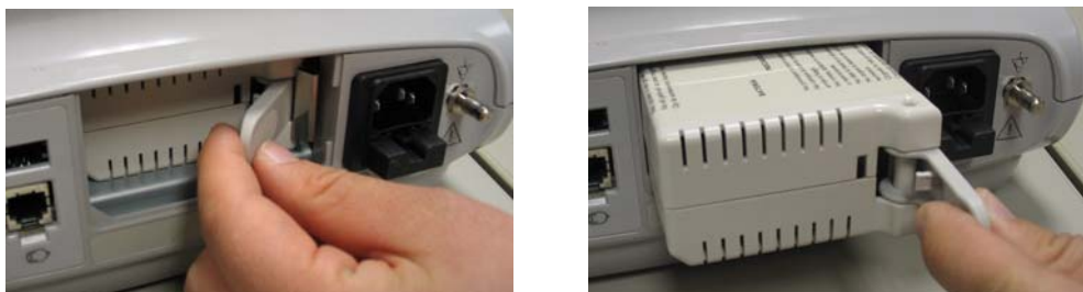
Figure 7-3 Removing the battery
