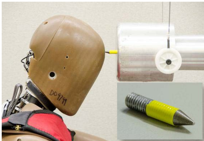
Figure 4-5. Use of a pointer tool to set impactor location
