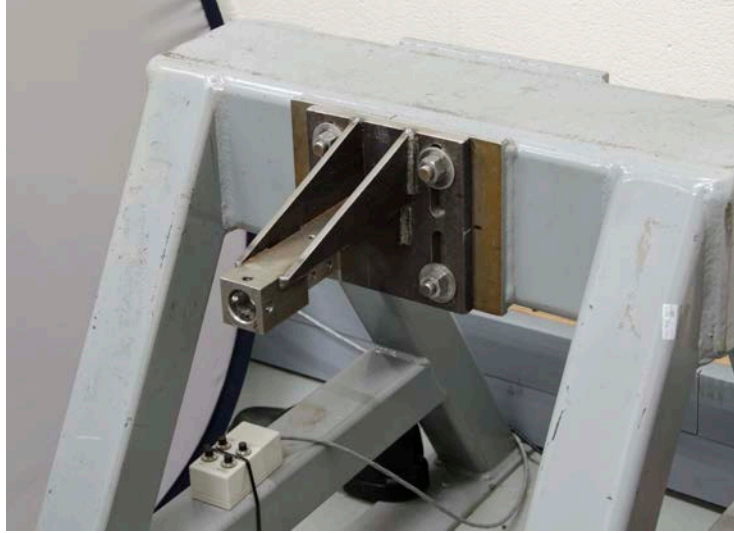
Figure 3-19. Install the lower leg mounting bracket
