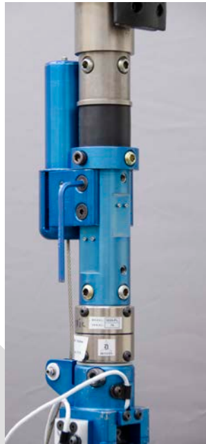
Figure 12-2. Remove Achilles spring tube assembly
