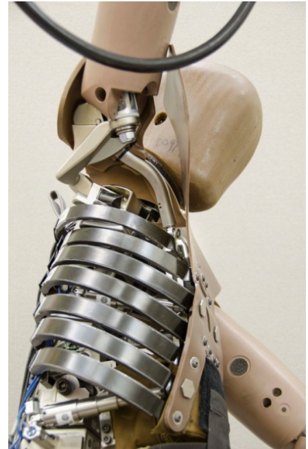
Figure 6-16. Rib #1 can be moved to access wiring for neck removal
