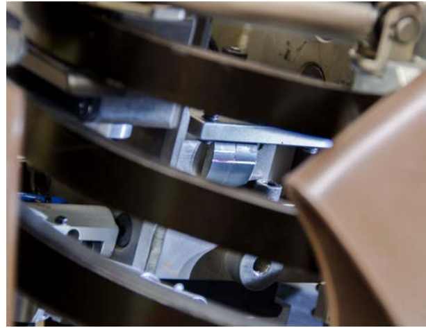
Figure 3-6. View of neck pitch change joint scribe lines through ribcage
