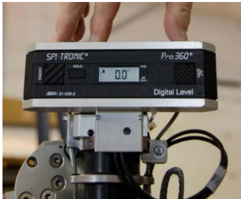
Figure 6-3. Inclinometer placement on top surface of upper neck load cell ( UpNeckLoadCell ° )
