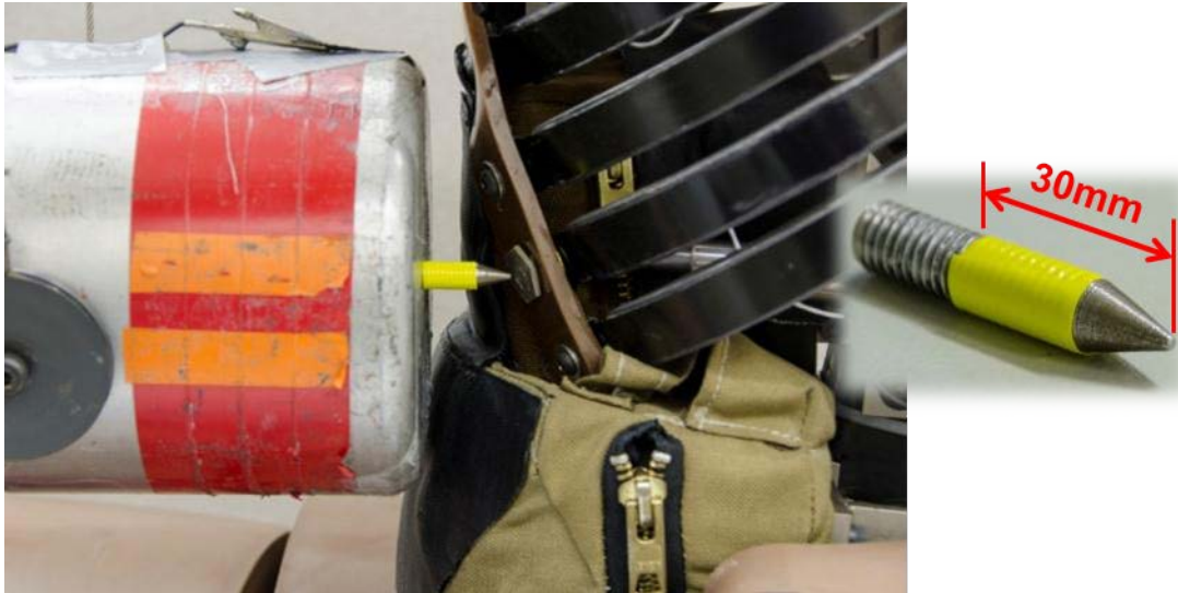
Figure 8-2. Alignment of impact location using pointer tool (shown in inset)
