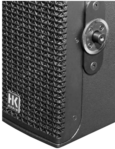
Figure 27 b: Attaching the MS/1 yoke to the CT 108
