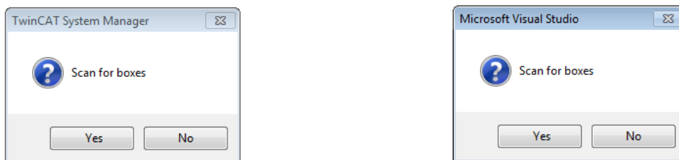
Fig. 95: Scan query after automatic creation of an EtherCAT device (left: TwinCAT 2; right: TwinCAT 3)
