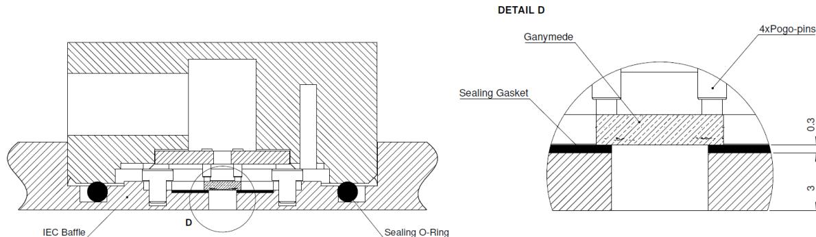
The outlet through the baffle for the speaker has the same shape as the inside of the speaker cover (4.99 x 3.01 mm with radius 1.2 mm).
