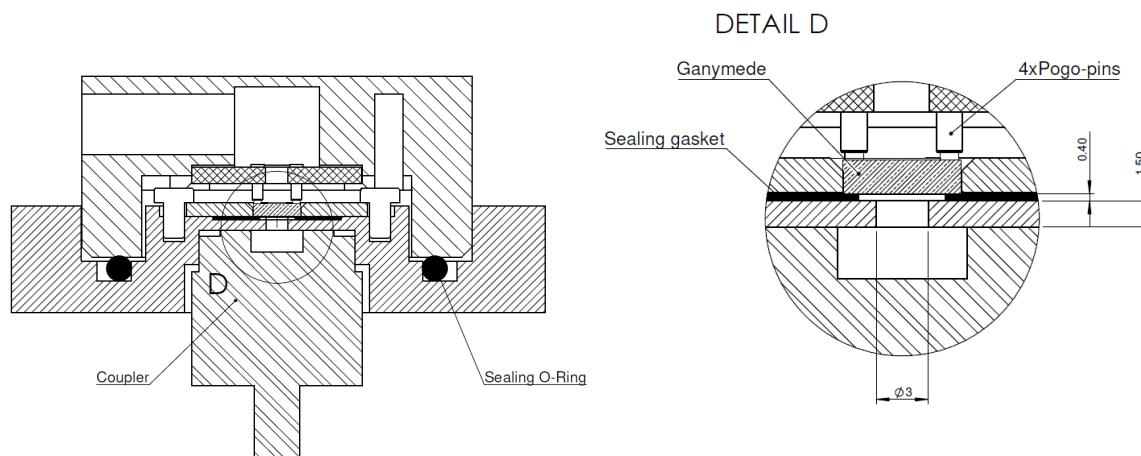
The outlet from the speaker to the coupler is round with a diameter of 3 mm.
