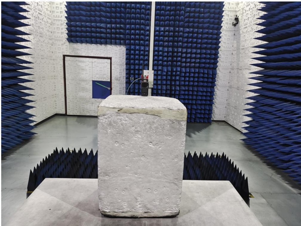
RADIATED EMISSION ABOVE 1G TEST SETUP
