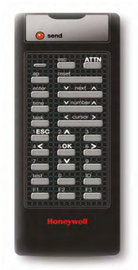
FIGURE 5-2 The key functions of the Fusion4 IR Controller
