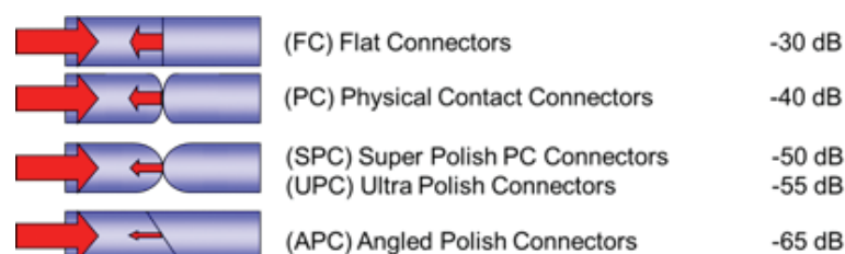
Figure 5. Typical connector types and reflectance values
