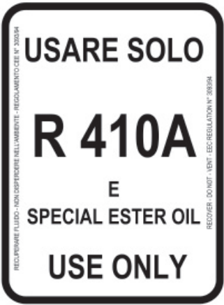
Identification of the refrigerant - External door
