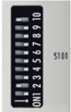
Fig. 19: DIP switch S001: Left off "0", right on "1"
