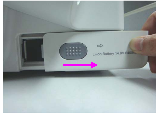
② Pull the battery compartment door out
