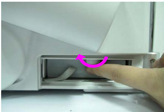
⑤ Turn the lever clockwise to keep the battery in place
