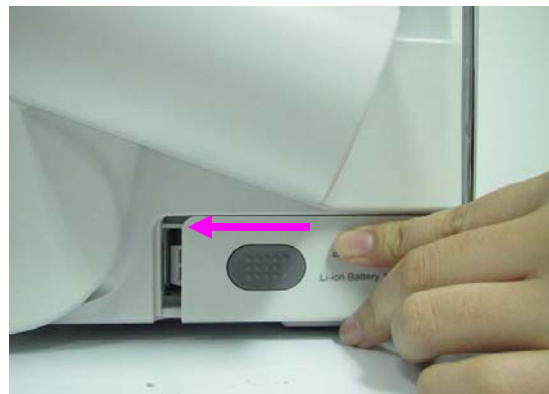
⑥ Replace the battery compartment door
