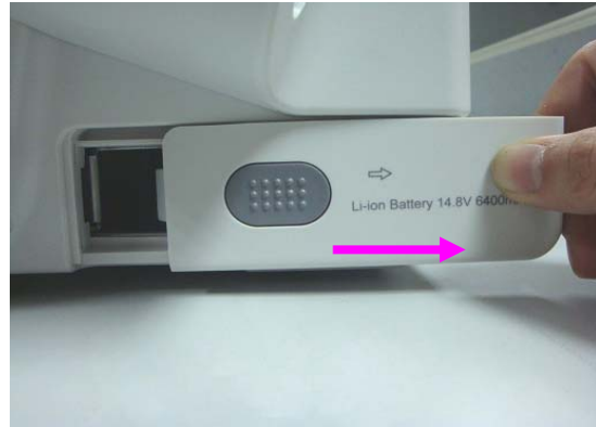
② Pull the battery compartment door out
