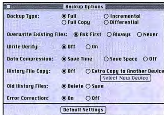
Fastback II offers a variety of backup options that you can save in configuration files for specific backup sessions.
