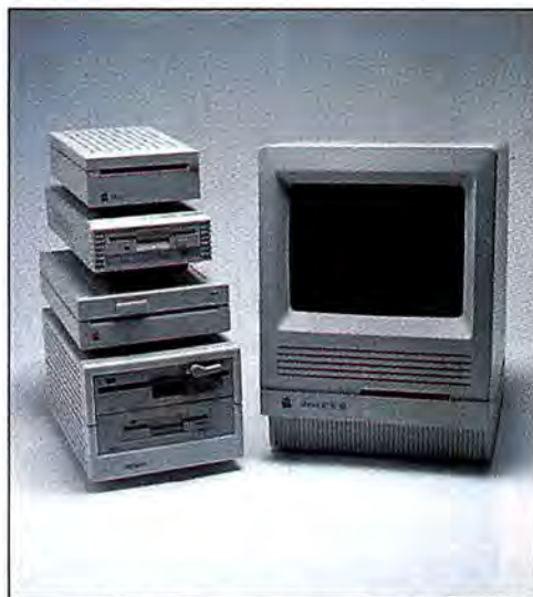
Figure 5: Five floppy drives that read DOS-formatted disks (starting bottom left, clockwise): This DaynaFile model reads both 5.25- and 3.5-inch DOS floppies and connects to the Mac's SCSI port. The Apple PC 5.25 connects to an expansion card on the Mac. PLI and Apple sell external versions of the FDHD found in the Mac SE/30, IICx, and IICx.
