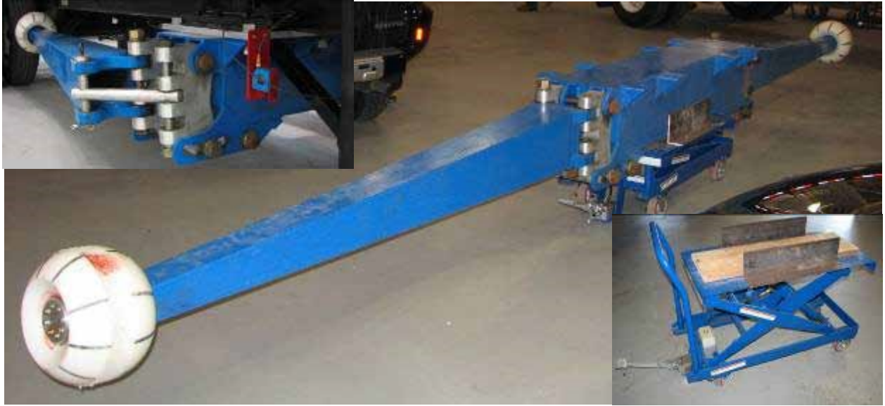
Figure 4.22: Center: completely assembled new NHTSA outriggers ready to go under a trailer. Top Left: picture of the outriggers in transport position. Lower Right: Zorin hydraulic elevating lift cart with payload capacity of 2000lbs and height range of 15.0 - 39.0 inches. It is used to ease the moving and installation of outriggers.
