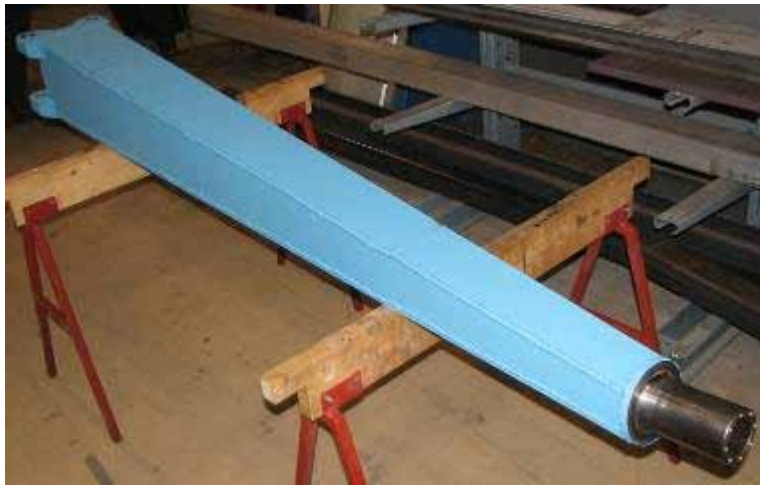
Figure 4.7: Finished welded and painted Outboard Beam.
