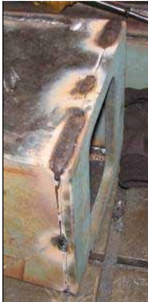
Figure 4.3: Left: Base Plate is added to the end. Middle: Base plate is welded to the Outboard Beam in the locations that the Hinge Brackets will overlap. Right: Hinge Brackets are being jigged up to weld. The bolts shown in the photo were removed and an aluminum jig was inserted into the holes to assure alignment, see Figure 4.4 (Middle).
