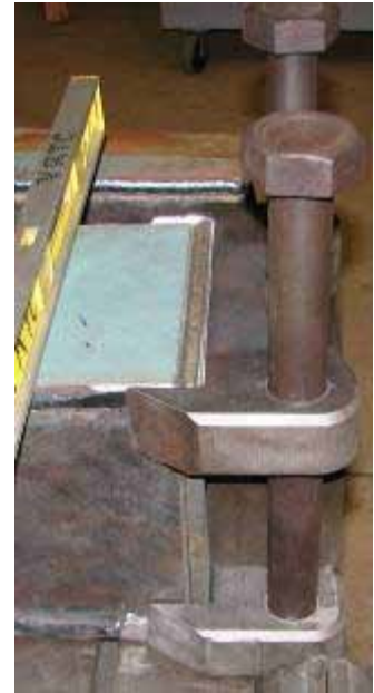
Figure 4.3: Left: Base Plate is added to the end. Middle: Base plate is welded to the Outboard Beam in the locations that the Hinge Brackets will overlap. Right: Hinge Brackets are being jigged up to weld. The bolts shown in the photo were removed and an aluminum jig was inserted into the holes to assure alignment, see Figure 4.4 (Middle).
