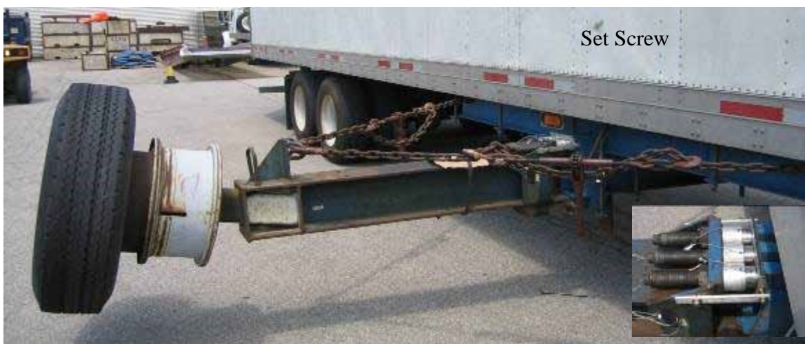
Figure 2.1: UMTRI trailer centrally mounted outriggers. Outrigger height is controlled with 3 large set screws indicated in the figure above.
