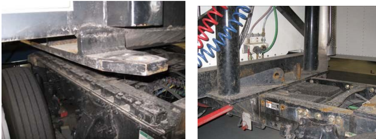
Figure B.2. Anti-jackknife mounts on tractor and trailer
