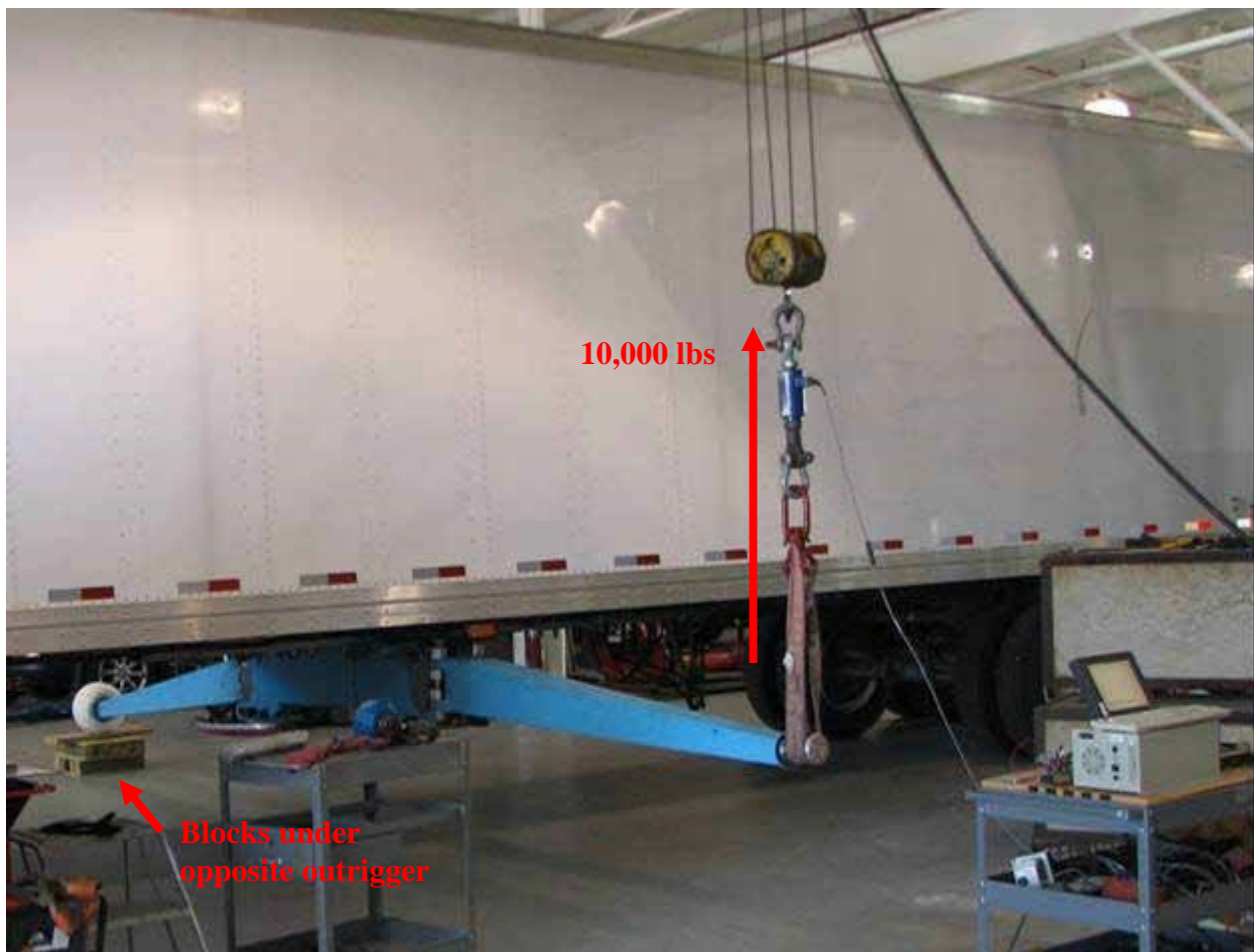
Figure 5.3: Static outrigger and outrigger mount load rating check. Wheel on opposite side is blocked so that both Outboard Beams are evaluated at the same time. The blocks were then removed and a load was reapplied to the
