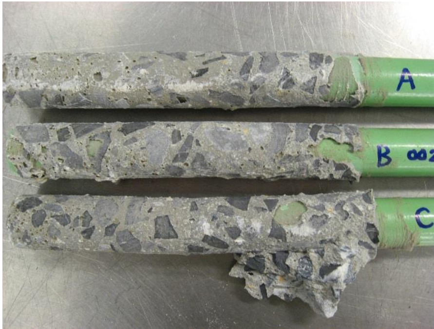
(Figure 5 – Examples of samples showing minimal unbonded areas)
