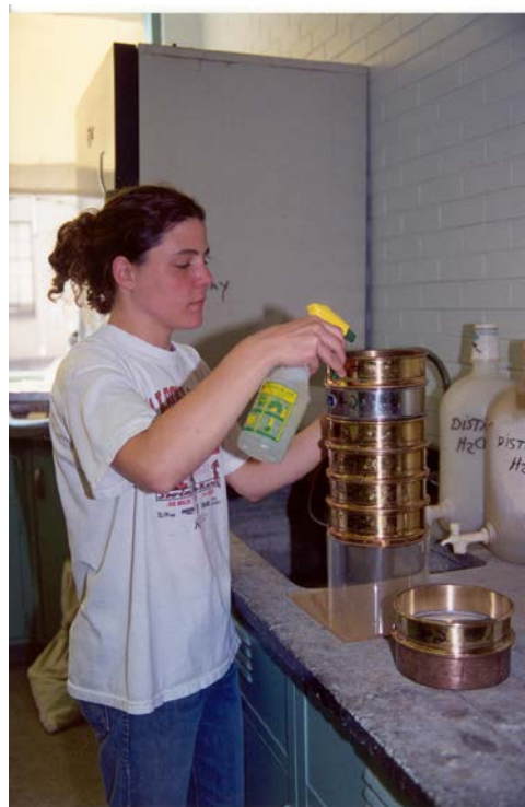
Figure 3- A 152.4 mm (6-inch) sieving cylinder connected to a sink aspirator, with the sieve stack assembled on top of the cylinder.
