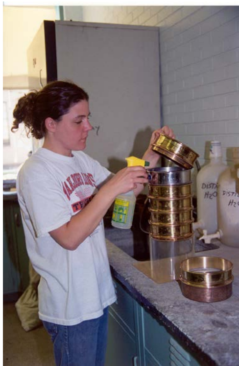
Figure 5- Spraying to clean off the interior of the sieve skirts
