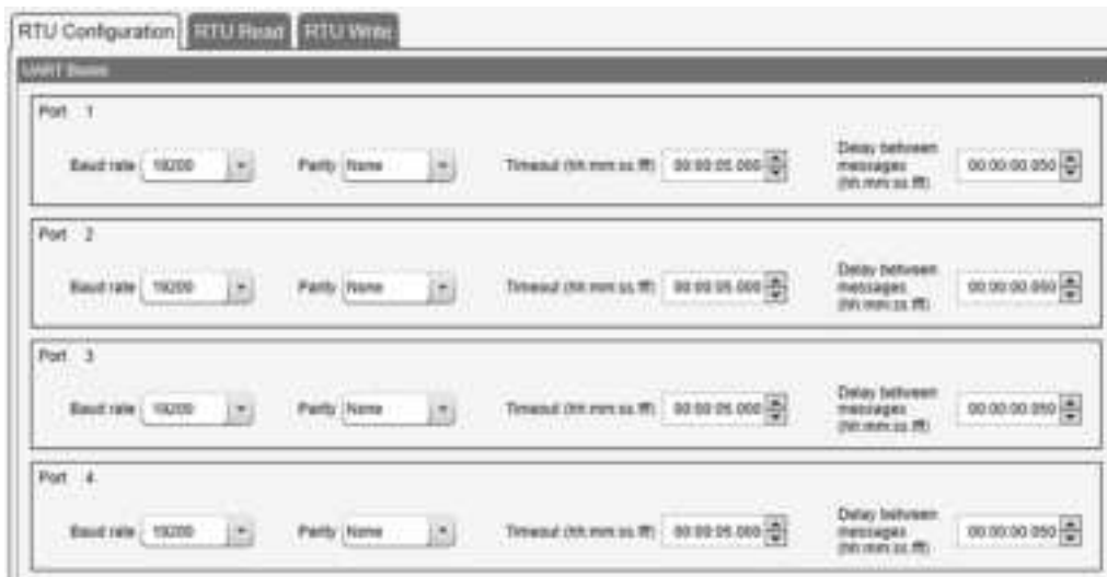
Figure 12. RTU Configuration screen for ports 0-4
