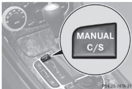
Program mode selector switch on SL 65 AMG
