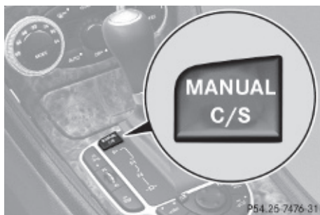
Program mode selector switch on SL 65 AMG
