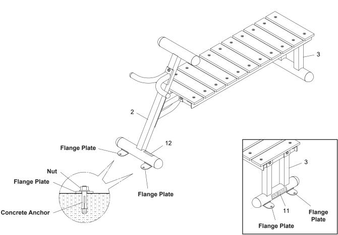
NOTE: Four concrete anchors (mounting hardware not included) are needed to secure the FRONT SUPPORT(2) and REAR SUPPORT(3) of the STAMINA® Outdoor Bench, two on each.
