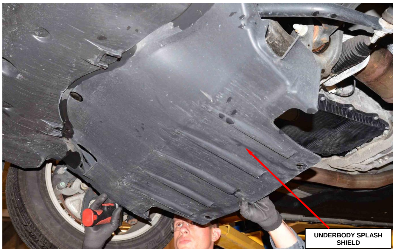
Figure 4 – Underbody Splash Shield
