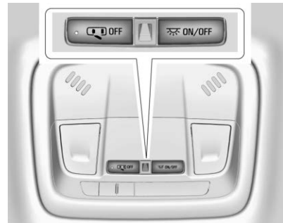
Dome Lamp Controls
