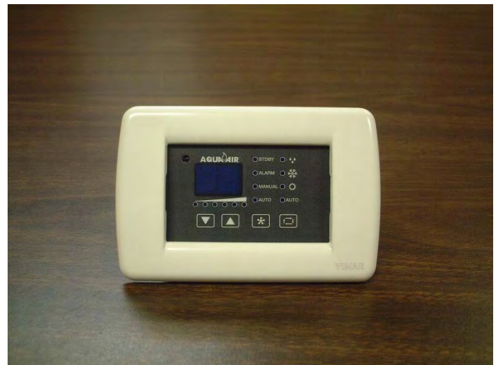
Vimar Bezel after installation on Sapphire TSV-01 Display Head
