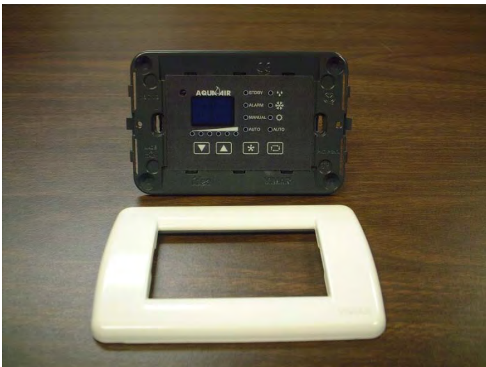
Vimar Bezel before installation on Sapphire TSV-01 Display Head
