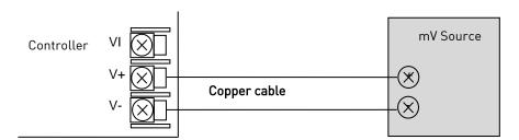
Ensure that no offsets have been set in the controller (see sections 4.6.2. – parameter **aF5**). Also ensure that no Two Point Offsets have been performed. If these adjustments *have* taken place, clear these settings before starting this procedure (see sections 4.6.2. – parameter **aF5** and section 4.8 – **ucAL**).
