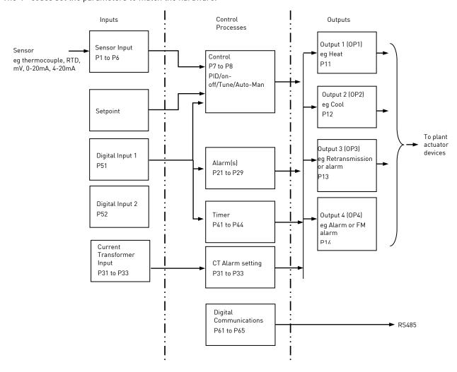
The Temperature (or Process Value, PV) is measured by the sensor and compared with a Setpoint (SP) set by the user.
