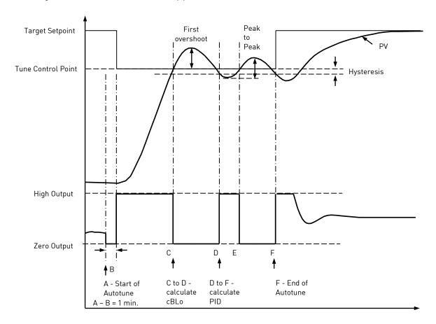
For a tune from below setpoint 'cbLa' is calculated on the basis of the size of the overshoot (assuming it was not set to Auto in the initial conditions). cbH is then set to the same value as cbLa.
