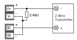
All models using an external power supply
