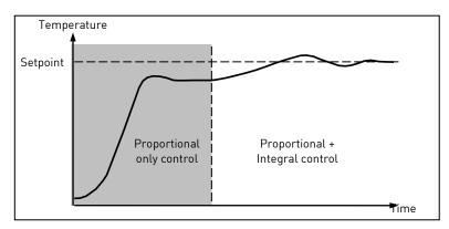
The units for the integral term are measured in time (1 to 9999 seconds). The longer the integral time constant, the more slowly the output is shifted and results in a sluggish response. Too small an integral time will cause the process to overshoot and even oscillate. The integral action may be disabled by setting its value to OFF.
