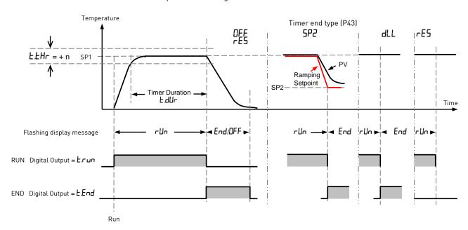
**Notes**: The dwell period can be reduced or increased while the timer is running by adjusting  $\mathcal{E}_{\mathcal{F}}\mathcal{E}$  (Time Remaining) in Level 2.
