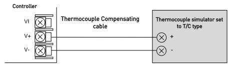
Set the mV source to the same thermocouple type as that configured in the controller.
