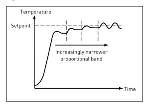
The diagram also shows the effect of narrowing proportional band to the point of oscillation. A very wide proportional band results in straight line control but with an appreciable initial error between setpoint and actual temperature. As the band is narrowed the temperature gets closer to setpoint. If the proportional band is very narrow the loop becomes unstable resulting in an oscillatory response.
