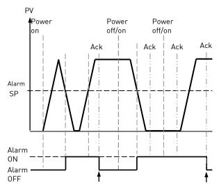
**Note**: The alarm will only cancel when the alarm condition is no longer current AND then it is acknowledged
