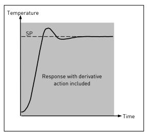
The derivative modifies the output to reduce the rate of change of error. It reacts to changes in the PV by changing the output to remove the transient. Increasing the derivative time will reduce the settling time of the loop after a transient change.
