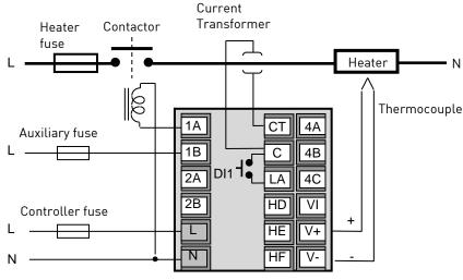
**Note**: a burden resistor value  $10\Omega$  is mounted inside the controller.
