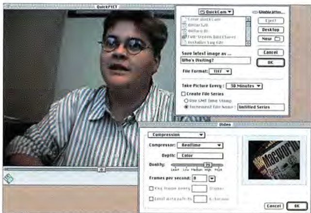
The Color QuickCam takes decent-quality images even at half-screen resolution (320 by 240 pixels), although the frame rate suffers.
