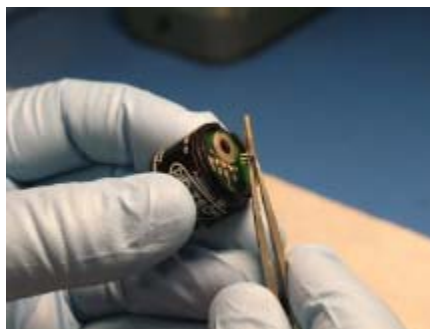
Figure 7–12. Installing the Cell Assembly
