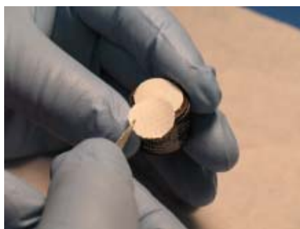
Figure 7-14. Placing the Filter Media
