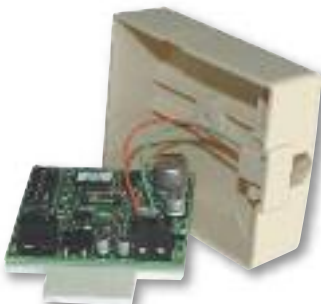
Model TR-1 (shown open) are concealed in a standard RJ-11 Jack.
