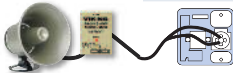
Maximum distance from M2W to paging horn is 250 feet.
