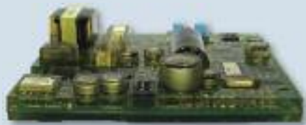
Tough and durable thermoplastic potting
