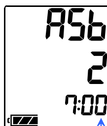
2nd start time of alarm
