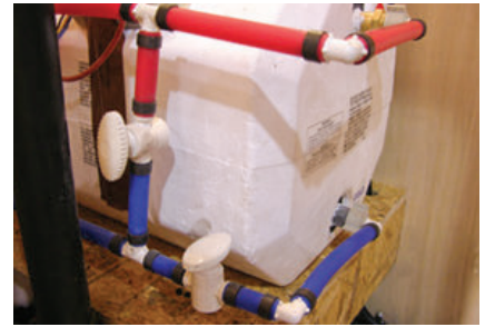
Flush the water system with fresh water before opening the bypass valves on the water heater to eliminate any residual antifreeze in the system. Consider flushing the water heater before reinstalling the drain plug on the outside of the motorhome.
