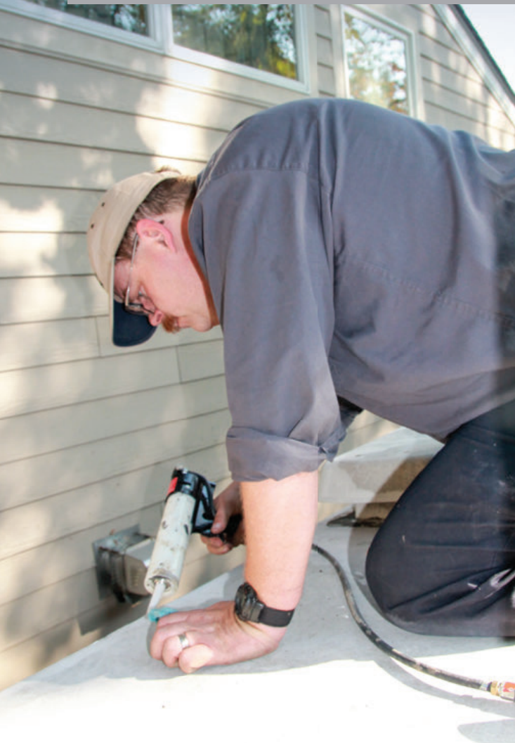
Spring is the optimal time to clean and reseal the roof of your motorhome. Be sure to use the proper sealant for the roof type.
