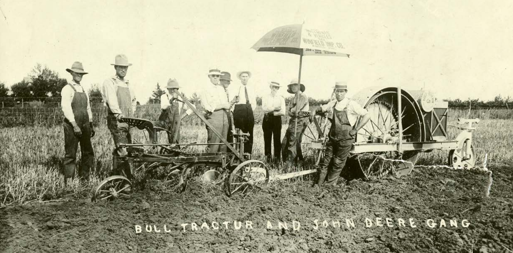
Testing of a John Deere Gang Plow with a Bull Tractor, 1912
