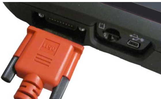
Figure 4-1 DA-4 data cable (26-pin end) connection to diagnostic tool
