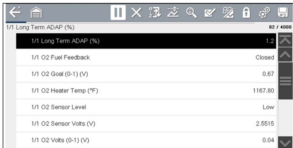
Figure 5-21 Data display (Typical - PID List view)
