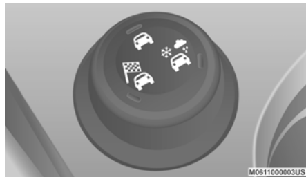
Dynamic Selector Switch
