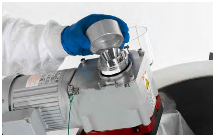
Figure 3.14. Removing the motor cap.
