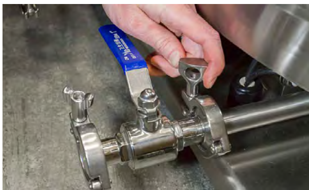
Figure 2.4. Attaching water jacket port using tri-clamp.
