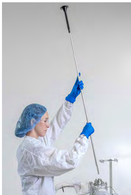
Figure 3.15. Loading drive shaft.
