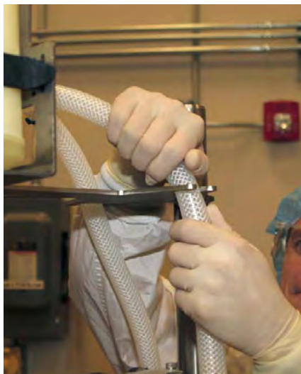
Figure 3.84. Clipping gas lines into place.
