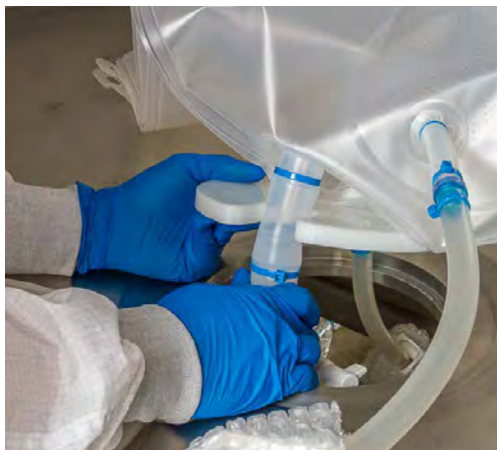
Figure 3.71. Drain line support.
