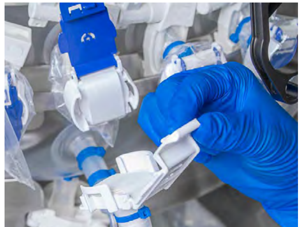
Figure 3.113. Opening protective cover pull tab on lineset.
