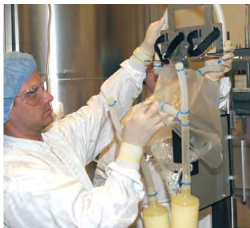
Figure 3.78. Routing gas inlet lines.
