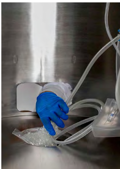
Figure 3.34. Sparge line insertion.
