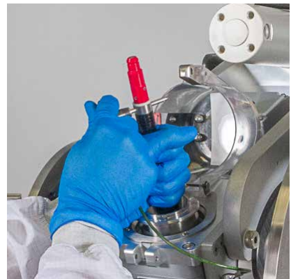
Figure 3.92. Using the latch pin.
