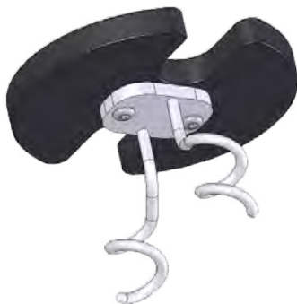
Figure 1.22. Sparge line support.
