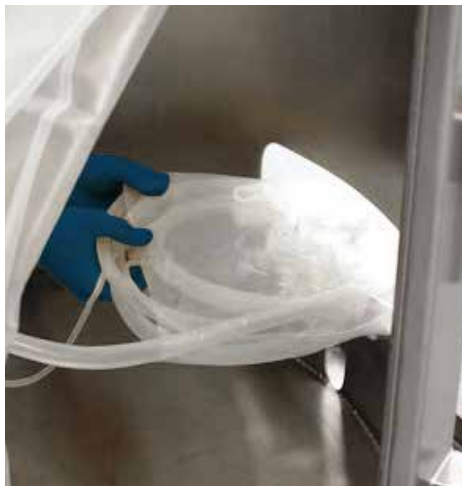
Figure 3.36. Drain/sampling line set insertion.
