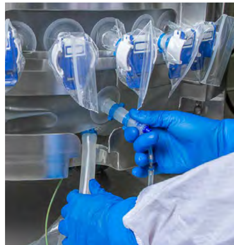
Figure 3.37. Drain/sampling line extension.
