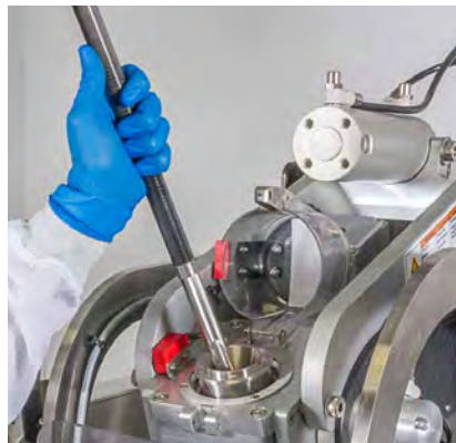
Figure 3.91. Insertion of the lower section of the drive shaft.
