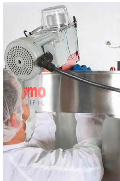
Figure 3.30. Bearing port orientation.
