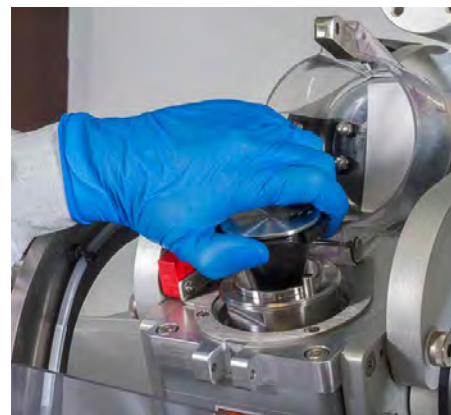
Figure 3.99. Engaging the bearing port.
