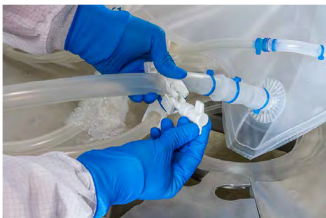
Figure 3.70. Clamping bottom drain line.
