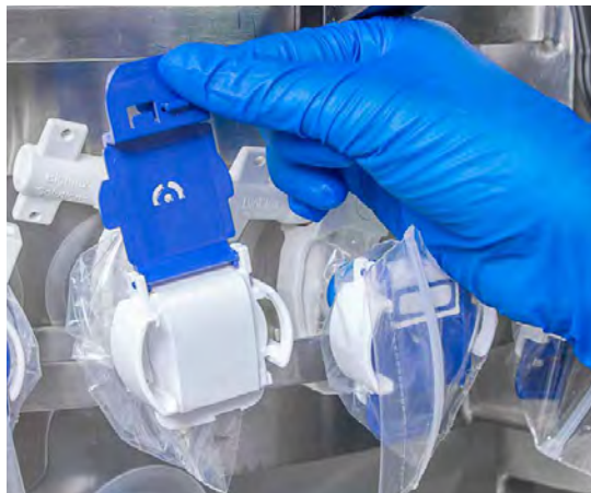
Figure 3.112. Opening protective cover pull tab on port.
