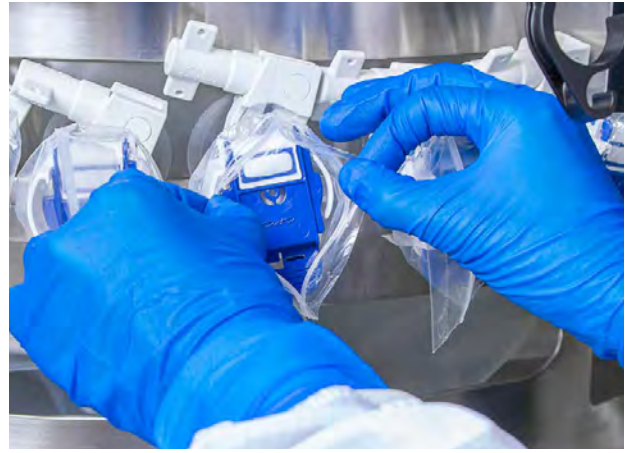
Figure 3.111. Removing plastic covering from connector.
