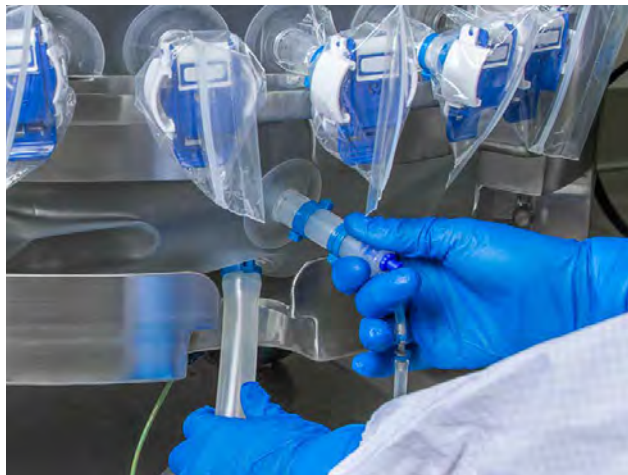
Figure 3.6. Drain line and port setup.
