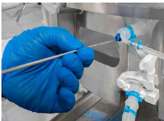
Figure 3.55. Temperature sensor insertion.
