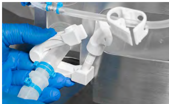
Figure 3.24. Bar clamp installation.
