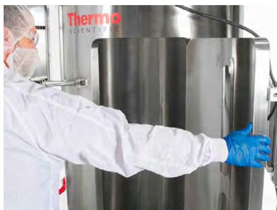
Figure 3.27. Opening the bioreactor door.
