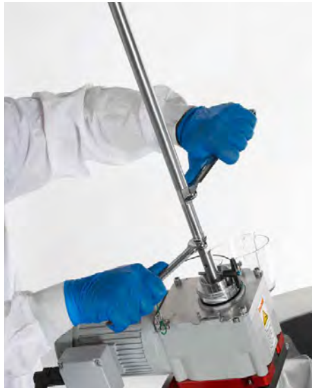
Figure 3.48. Tightening of shaft connections.
