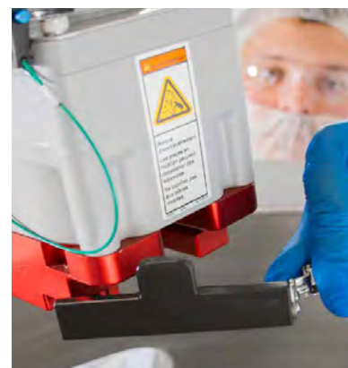
Figure 3.28. Close-up of bearing receiver clamp.
