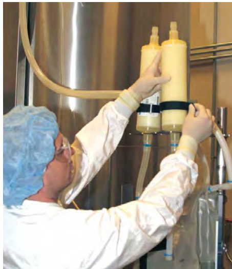
Figure 3.80. Securing vent filters.
