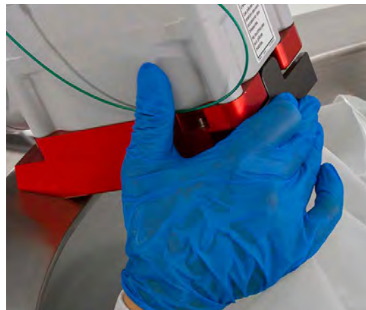
Figure 3.33. Door clamped shut.
