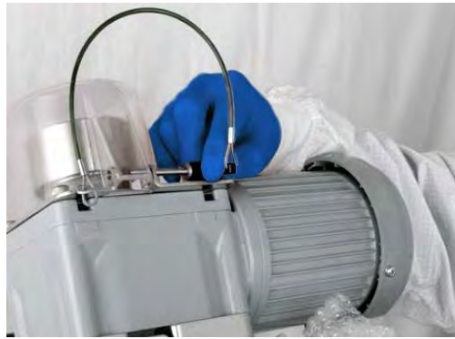
Figure 3.21. Replacing and latching cover.
