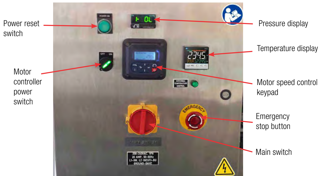
Figure 3.120. Front view of E-Box for 50–2,000 L S.U.B.s.
