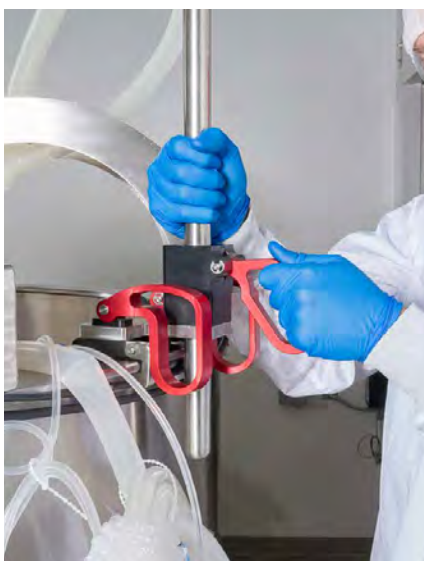
Figure 3.67. Raising the vent holder bracket.
