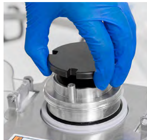
Figure 3.18. Drive shaft head aligned.
