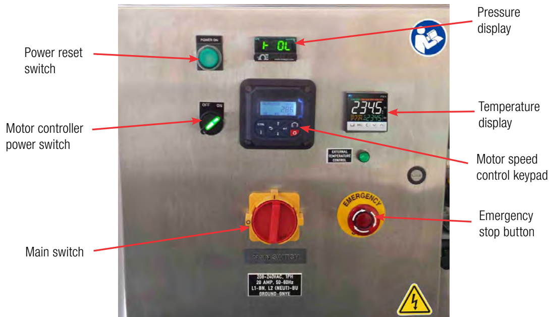
Figure 4.21. Front view of the E-Box for 50–2,000 L S.U.B.s.
