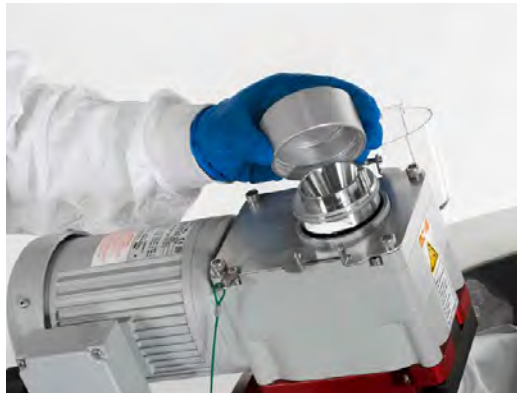
Figure 3.44. Latch pin removal.
