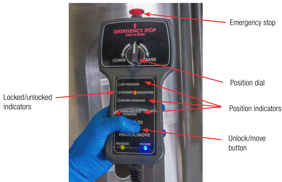
Figure 2.8. Handheld controller for motor lifts.
