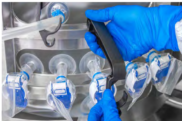
Figure 3.116. Attaching plastic probe clip.
