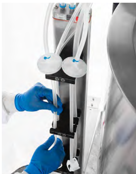
Figure 3.9. Inserting lines into the cable management system channels.
