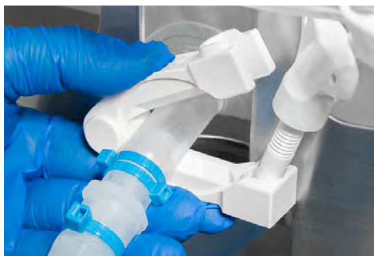
Figure 1.23. Heavy-duty tubing clamps.
