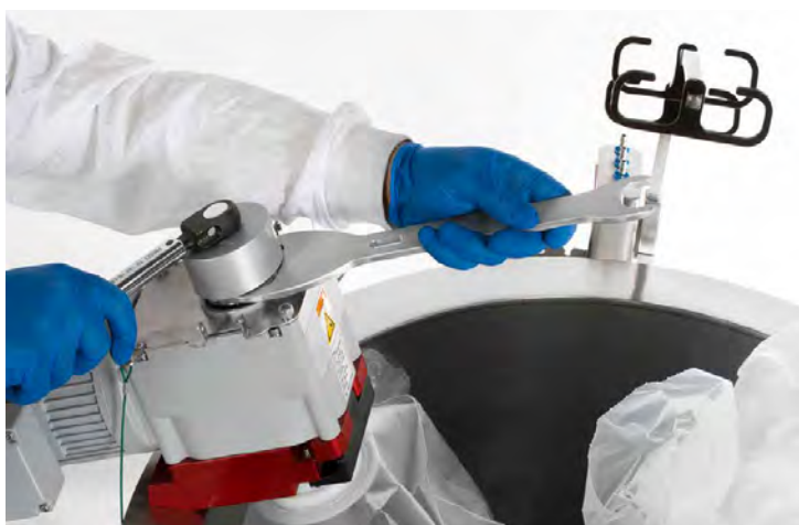
Figure 3.51. Tightening motor cap with wrenches.
