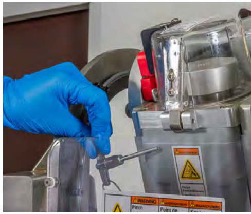
Figure 3.89. Removing latch pin.
