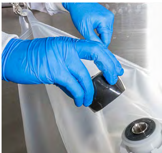
Figure 3.61. Removing the bearing port cap.
