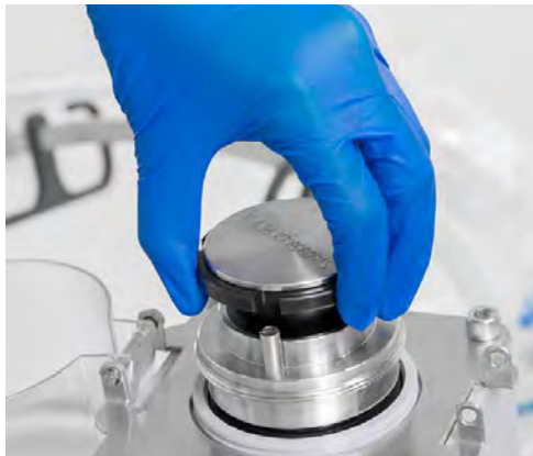
Figure 3.50. Drive shaft head aligned.
