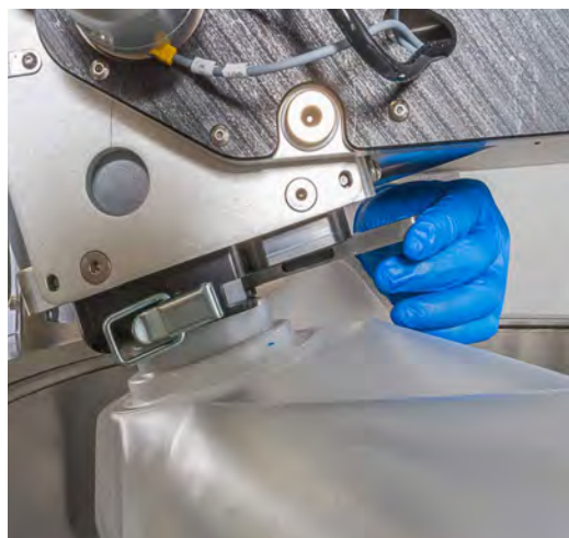
Figure 3.63. Closing and latching door.
