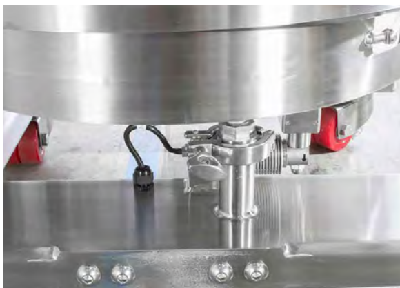
Figure 1.20. Load cell location.
