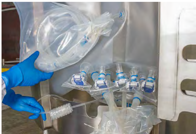
Figure 3.69. Feeding lines through the front access door.
