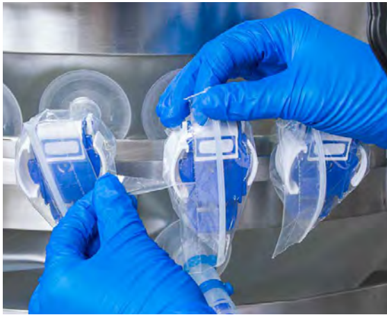
Figure 3.110. Pulling the tear strip.
