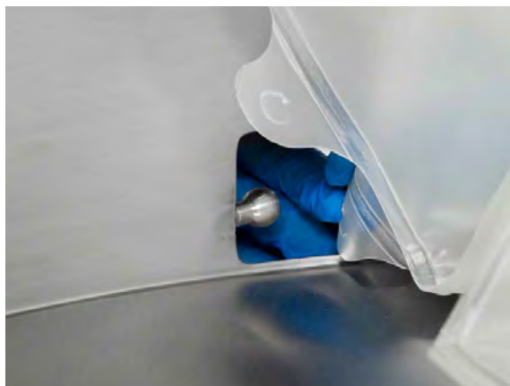
Figure 3.10. Attaching hanging tab and hook.
