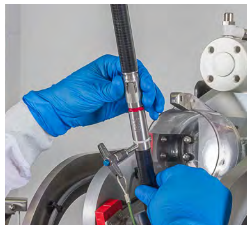
Figure 3.96. Red indicator ring exposed.
