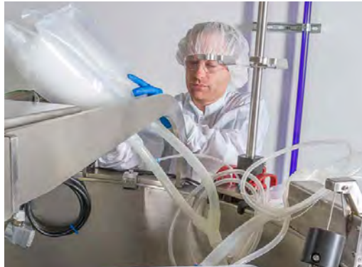
Figure 3.64. Placing linesets over tank edge.
