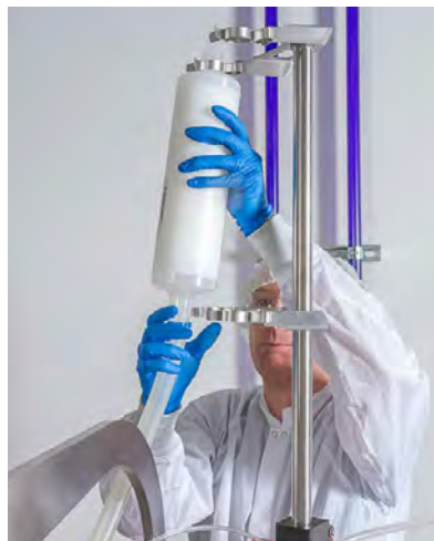
Figure 3.65. Clipping filter to holder.
