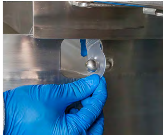
Figure 3.74. Securing the container tab on the pin.
