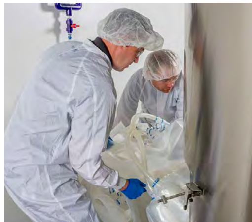
Figure 3.59. Loading the BPC.
