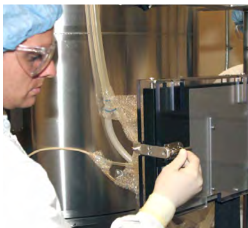
Figure 3.77. Opening the chiller plate doors.
