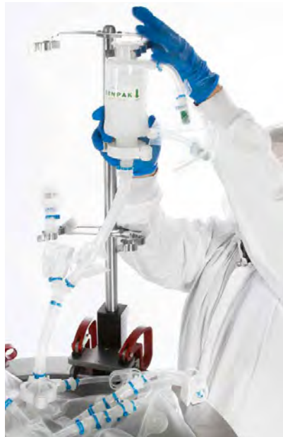
Figure 3.22. Vent filter installation.
