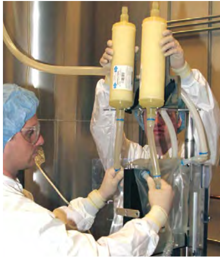
Figure 3.79. Placing vent filters.
