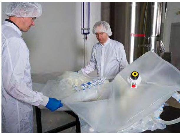
Figure 3.58. Removing the BPC from polybags.
