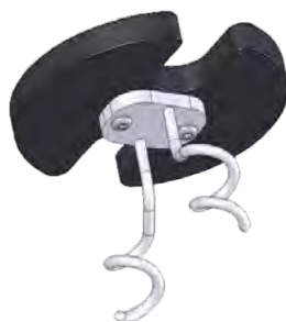
Figure 2.6. Sparge line support.
