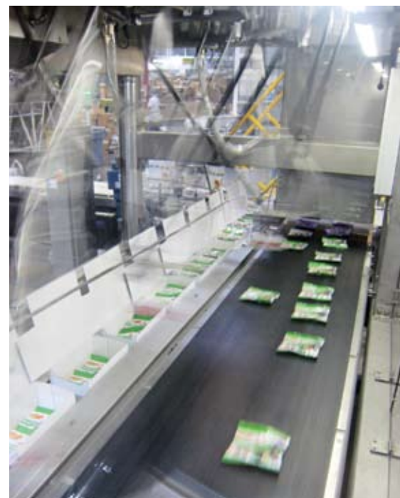
Three pick-and-place robots pick up bags of jelly beans from the incoming conveyor and place them into cartons. The system incorporates a vision system that locates the bags and directs the robots.
