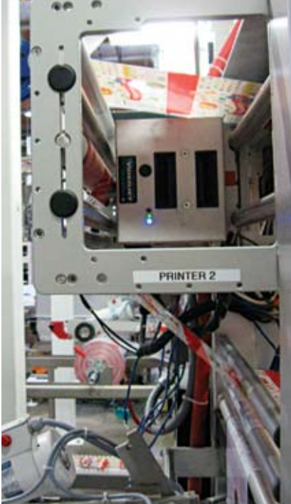
Two thermal-transfer printers print selected information on the film as it travels up the back of the vertical form/fill/seal machine, above. Operator stations are mounted next to the machines, below, for easy access.
