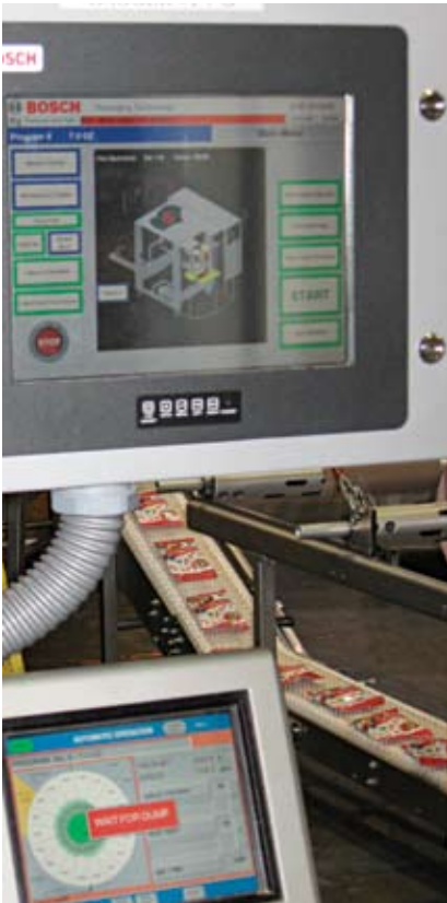
Two thermal-transfer printers print selected information on the film as it travels up the back of the vertical form/fill/seal machine, above. Operator stations are mounted next to the machines, below, for easy access.
