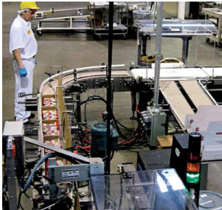
Cartons are formed from blanks, above, and are then delivered to the robotic case packer. Filled cartons from the packer travel over a checkweigher before they enter the closer, left.
