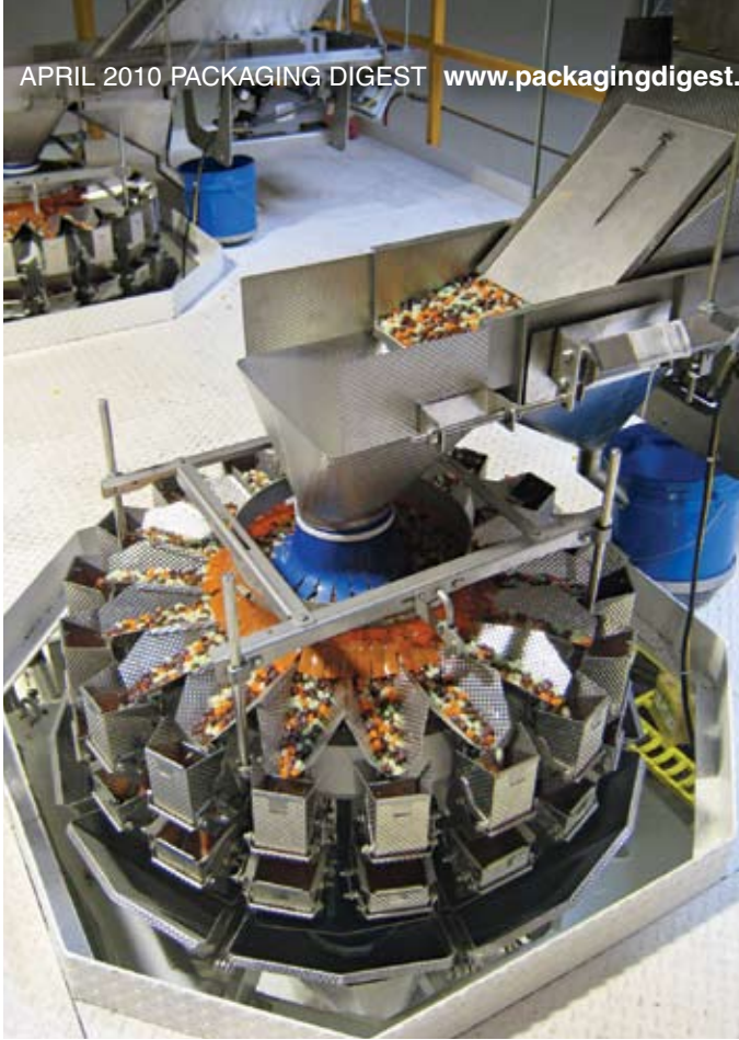
Two radial weighing systems, above left, feature 18 individual weigh heads each to keep up with the speed of the vertical form/fill/seal machines, above right. Jelly Belly beans discharge through metal detectors installed between the scales and the bag machines and continue into the bags being produced below.
