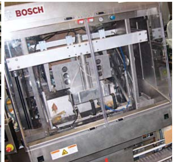
Cartons are formed from blanks, above, and are then delivered to the robotic case packer. Filled cartons from the packer travel over a checkweigher before they enter the closer, left.
