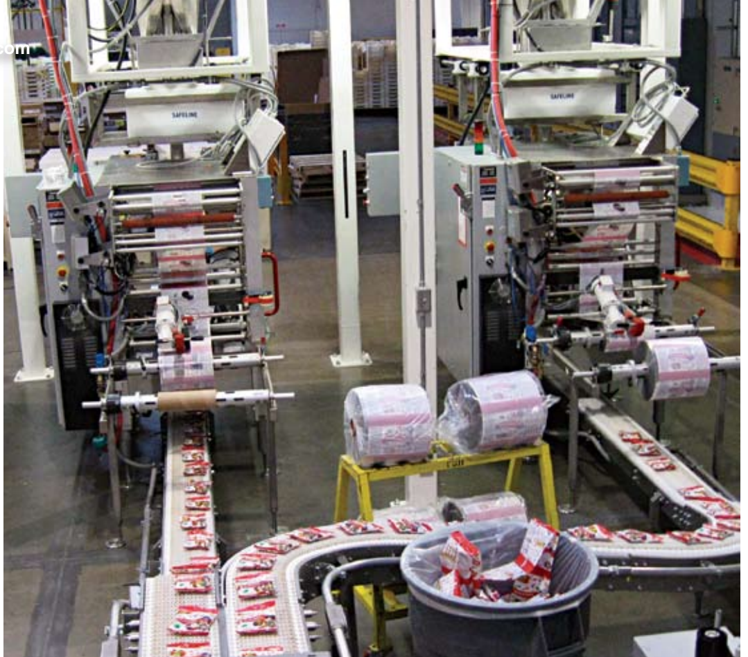
Two radial weighing systems, above left, feature 18 individual weigh heads each to keep up with the speed of the vertical form/fill/seal machines, above right. Jelly Belly beans discharge through metal detectors installed between the scales and the bag machines and continue into the bags being produced below.
