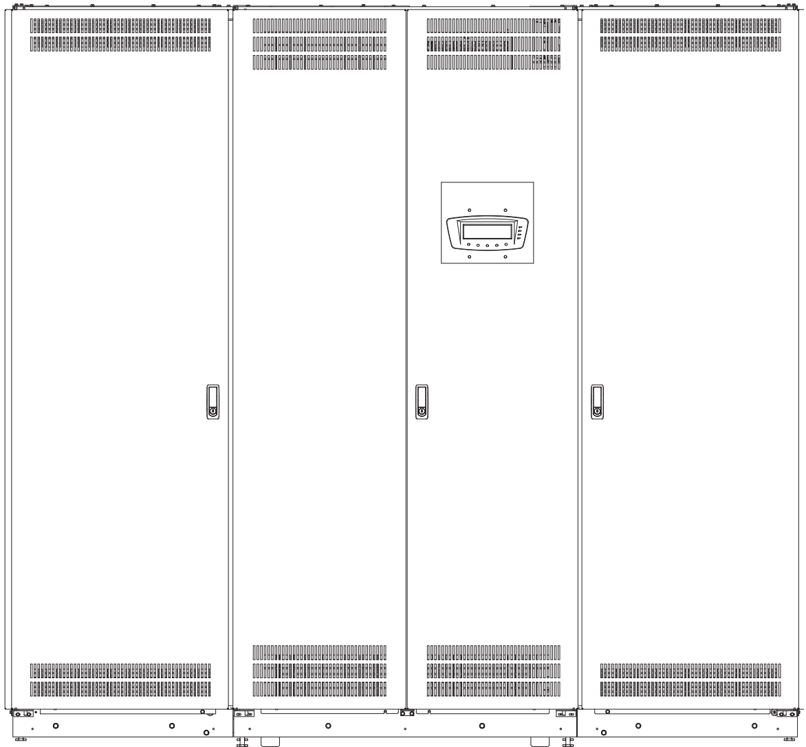
Figure 1-2. Eaton 150 kVA Three-Phase PDU Cabinet with Left and Right Front-Facing Sidecars
